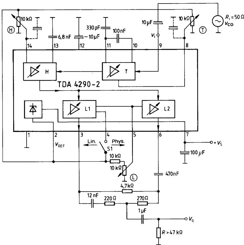
**Measurement circuit 2 (stereo operation)**
